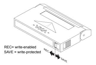
**Figure 3-3** Setting the write-protect switch
